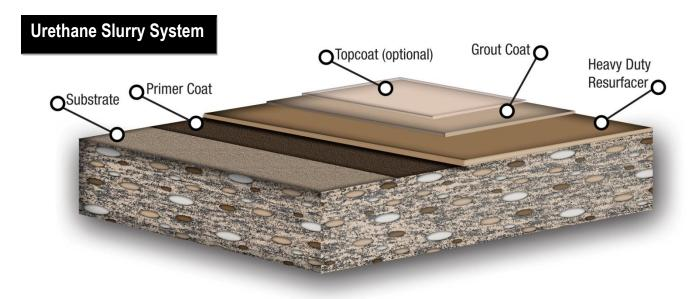
RS-31US is a Water-Based Cement Urethane Slurry Flooring System is a high heat resistant, high strength concrete resurfacing material. The versatility allows use in industries from food and beverage processing to chemical and water treatment facilities requiring a USDA compliant, thermal shock resistant grade floor or when a concrete floor has sustained damage requiring a 3/16" to 1/4" surface restoration.
